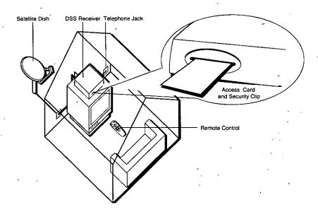
Satellite Dish Picks up the satellite's coded program information and relays it to your satellite receiver. (Your satellite dish may be installed in different locations on or around your house. The satellite dish must, however, be pointed in a southern direction toward the satellite.)
